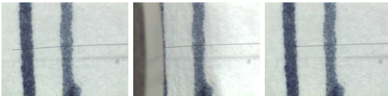
Figure 2: Microscope images of the cutting procedure. Only the very end of the fiber is removed to achieve a fresh electrode surface.
